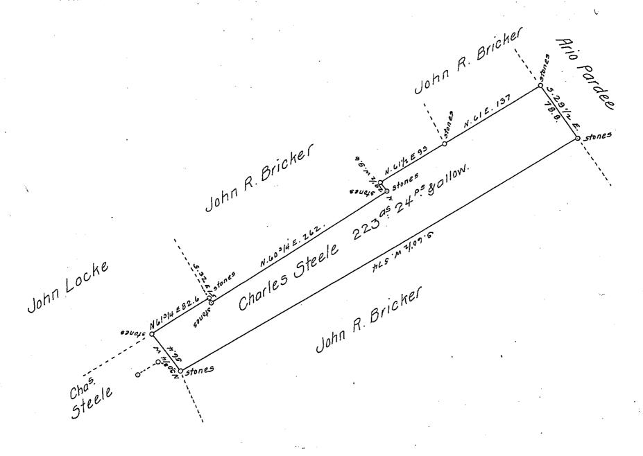
A draft of a Tract of Land, Situated in the Township of Armagh and County of Mifflin, containing two hundred and twenty-three acres, and twenty-four perches and allowance of Six per cent for Roads&c.
